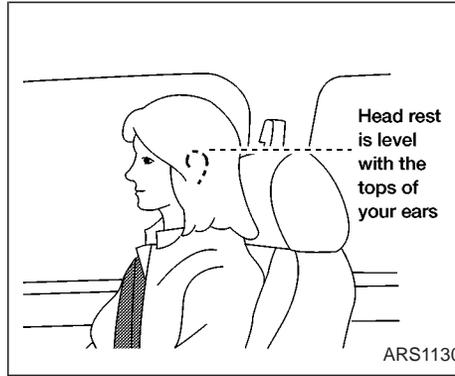
Adjust the top of the head restraint even with the tops of your ears.
